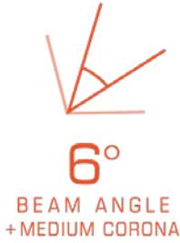
LED SOLARIS NEXT GEN is a universal primary dive light that is built to withstand the harshest underwater environments while reliably pumping out up to 4500 lumens of light that narrows to 6 degrees spot surrounded by a bright corona around the central beam.
